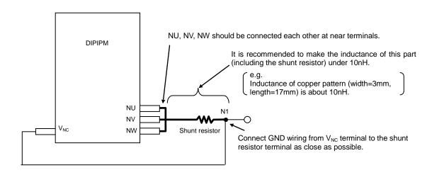
Fig.3-1-9 Wiring instruction (In the case of using with one shunt resistor)
