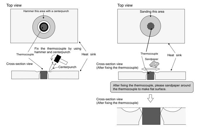
Fig. 3-2-5 Example of installation of thermocouple
