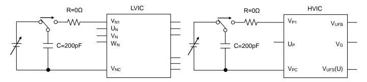
Fig.3-3-3 LVIC terminal Surge Test circuit
