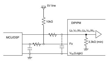
Fig.3-1-6 Control input connection
