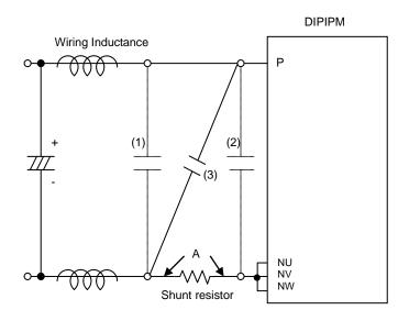
Fig.3-1-8 Recommended snubber circuit location
