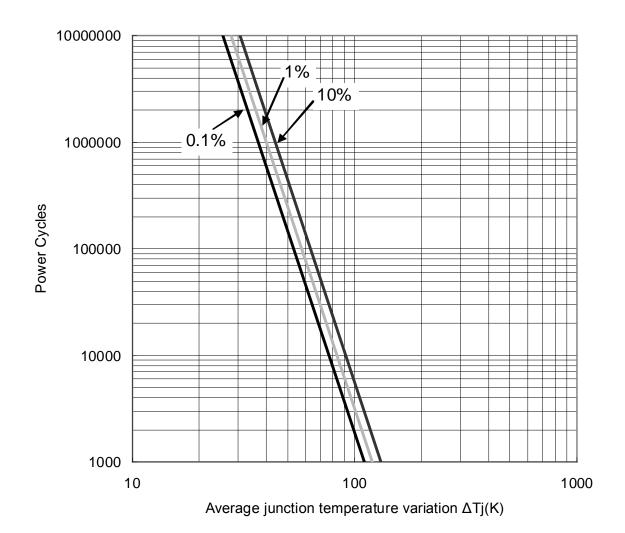
Fig.3-1-19 Power cycle curve
