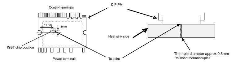
Fig. 3-2-4 Point for installing thermocouple in external heat sink
