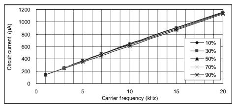
Fig.4-2-4 I<sub>DB</sub> vs. Carrier frequency for PSS20S92\*6-AG
