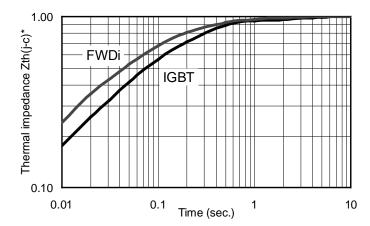
Fig.2-1-3 Typical transient thermal impedance
