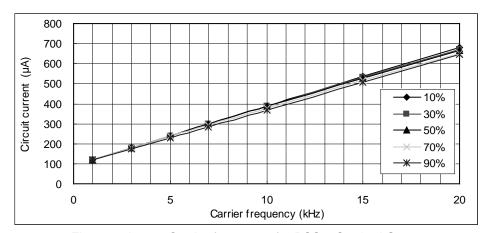
Fig.4-2-2 I<sub>DB</sub> vs. Carrier frequency for PSS10S92\*6-AG
