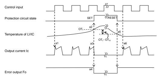
Fig.2-2-7 Timing Chart of OT protection
