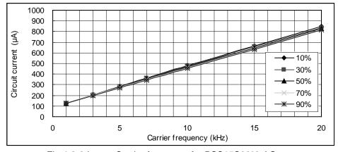
Fig.4-2-3 I<sub>DB</sub> vs. Carrier frequency for PSS15S92\*6-AG
