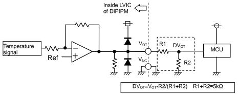
Fig.2-2-13 V<sub>OT</sub> output circuit in the case with high protection level
