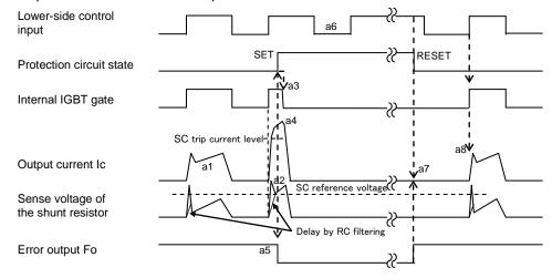
Fig.2-2-3 SC protection timing chart
