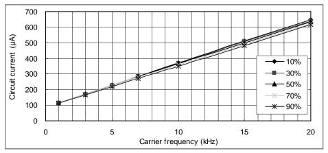
Fig.4-2-1 I<sub>DB</sub> vs. Carrier frequency for PSS05S92\*6-AG
