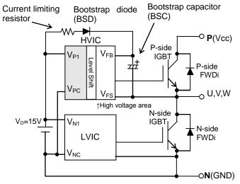
Fig.4-1-1 Bootstrap Circuit Diagram
