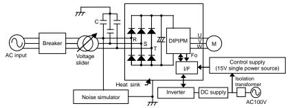
Fig.3-3-1 Noise withstand capability evaluation circuit
