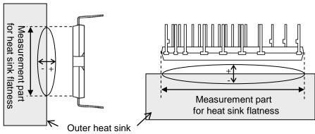
Fig.2-4-2 Measurement point of heat sink flatness
