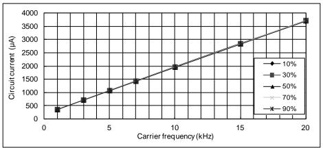
Fig.4-2-6 I<sub>DB</sub> vs. Carrier frequency for PSS35S92\*6-AG
