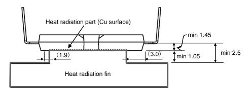
Fig.2-1-1 In the case of using convex fin (unit: mm)
