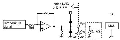
Fig.2-2-11 V<sub>OT</sub> output circuit in the case of detecting low temperature
