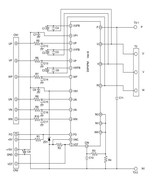
Fig.5-3-1 Demo board circuit schematic
