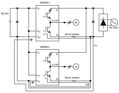
Fig.3-1-13 Parallel operation
