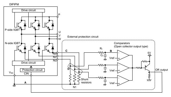
Fig.3-1-4 Interface circuit example
