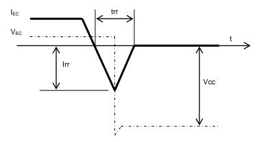
Fig.3-2-1 Ideal FWDi recovery characteristics curve
