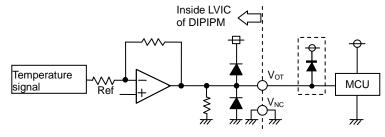
Fig.2-2-12 V<sub>OT</sub> output circuit in the case of using with low voltage controller
