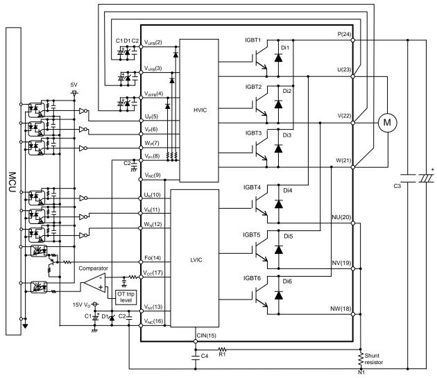
Fig.3-1-3 Interface circuit example with optocoupler
