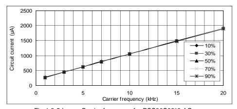
Fig.4-2-5 I<sub>DB</sub> vs. Carrier frequency for PSS30S92\*6-AG
