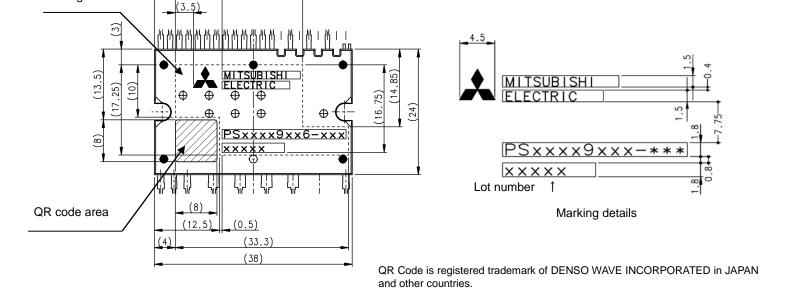
Fig.2-3-2 Laser marking view
