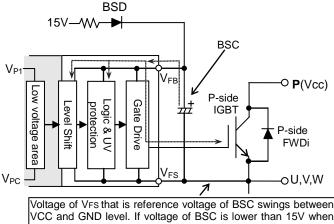
Voltage of VFs that is reference voltage of BSC swings between VCC and GND level. If voltage of BSC is lower than 15V when VFs becomes to GND potential, BSC is charged from 15V N-side control supply.
