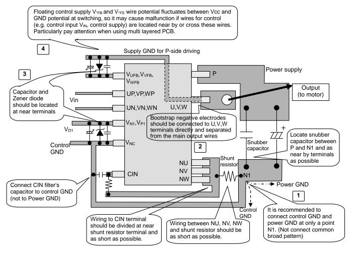
Fig.3-1-12 Precaution for wiring on PCB
