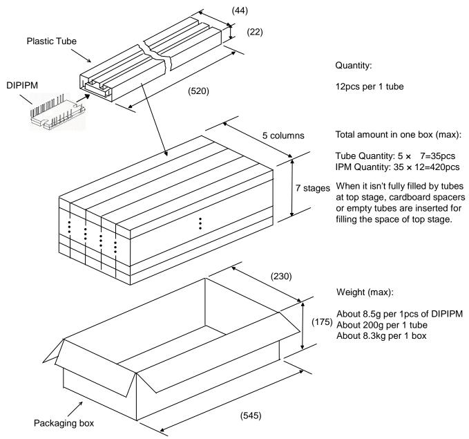
Spacers are put on the top and bottom of the box. If there is some space on top of the box, additional buffer materials are also inserted.
