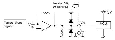
Fig.2-2-10 V<sub>OT</sub> output circuit
