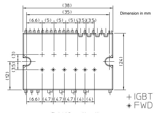
Fig.2-1-2 Power chip position
