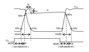
Fig.2-1-4 Switching time definition
