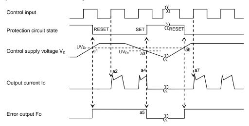
Fig.2-2-4 Timing chart of N-side UV protection
