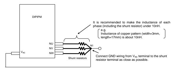
Fig.3-1-10 Wiring instruction (In the case of using with three shunt resistor)
