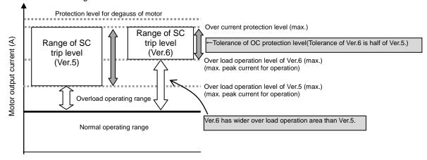
Fig.1-5-1 short circuit trip level
