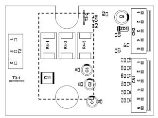
Fig.5-2-1 Demo board component layout (DIPIPM is mounted to back side.)
