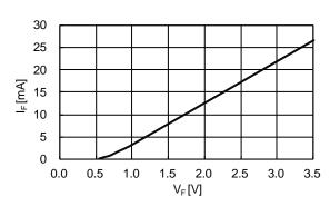
Fig.4-3-1 V<sub>F</sub>-I<sub>F</sub> curve for bootstrap Diode (rated current 5A~20A, the right figure is enlarged view)
