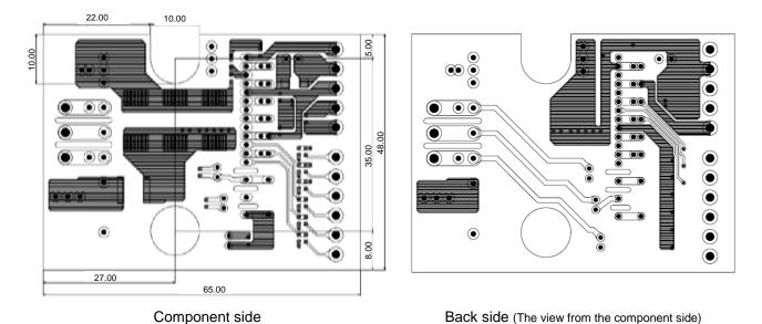
Fig.5-2-2 Demo board PCB pattern layout
