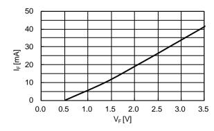
Fig.4-3-2 V<sub>F</sub>-I<sub>F</sub> curve for bootstrap Diode (rated current 30A, 35A, the right figure is enlarged view)
