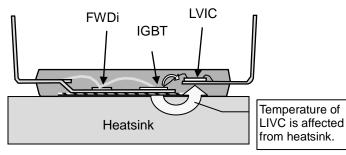
Fig.2-2-9 Thermal conducting from power chips
