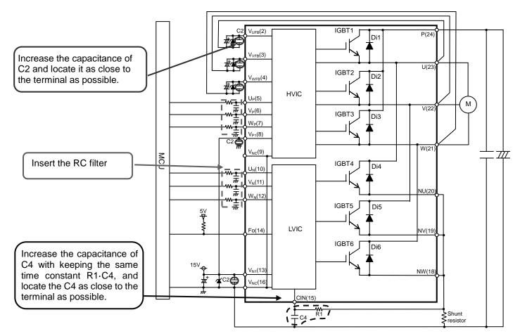
Fig.3-3-2 Example of countermeasures for inverter part
