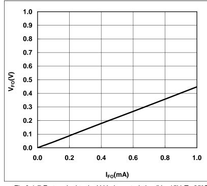
Fig.3-1-7 Fo terminal typical V-I characteristics (V<sub>D</sub>=15V, T<sub>i</sub>=25°C)
