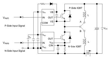
Fig.2-1-5 Evaluation circuit (inductive load)
