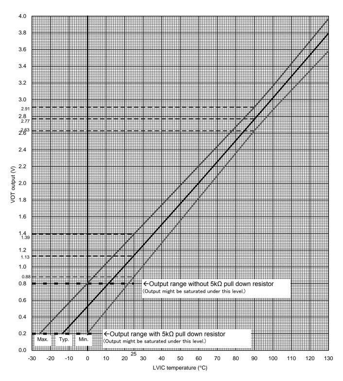
Fig.2-2-14 V<sub>OT</sub> output vs. LVIC temperature
