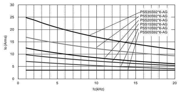
Fig.3-2-2 Effective current-carrier frequency characteristics
