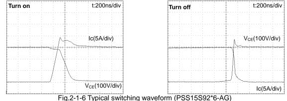
Conditions: V<sub>CC</sub>=300V, V<sub>D</sub>=V<sub>DB</sub>=15V, Tj=125°C, Ic=15A, Inductive load half-bridge circuit
