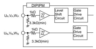
Fig.3-1-5 Internal structure of control input terminals
